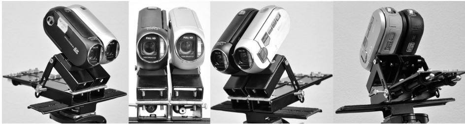
Figure 1: Stereoscopic camera system (source: authors)
