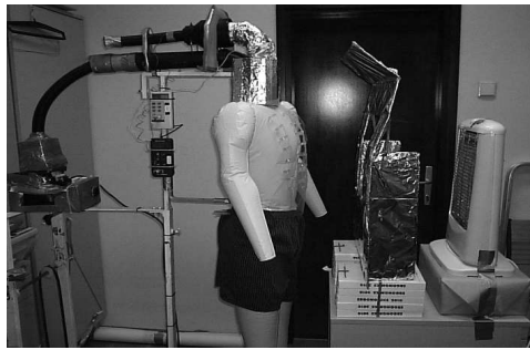
Figure 3. Inflatable thermal mannequin George ©
